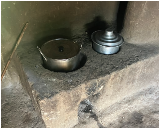
A fuel-efficient Lorena woodstove, which can significantly decrease fuelwood consumption and exposure to smoke among women. Photo: Sarah Juster
