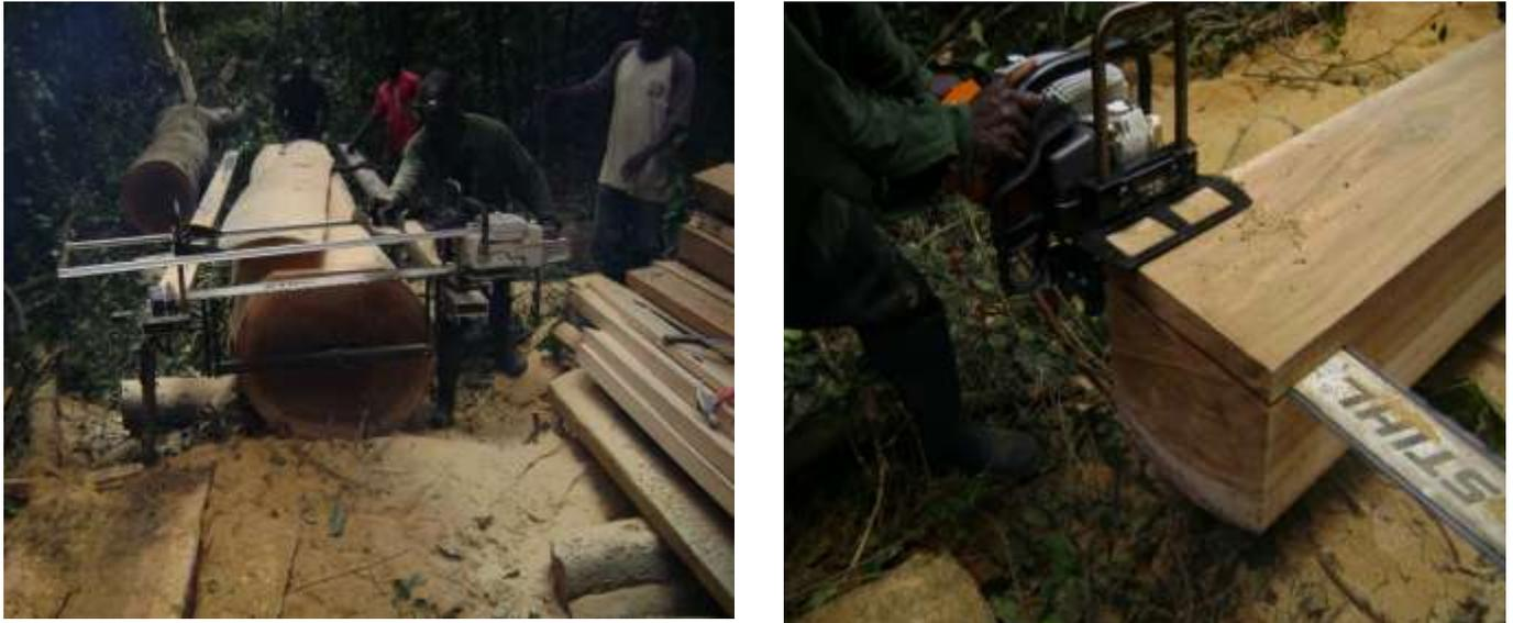
Figure1: Milling of logs using Logosol machines.
